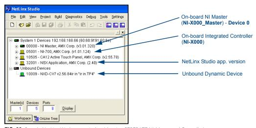
FIG. 30 Sample NetLinx Workspace window (showing SEPERATE NI-Master and Controller)
